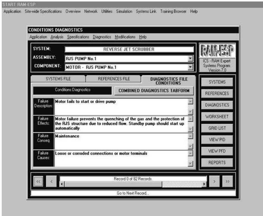
Fig. 3.67 Hazards criticality analysis assembly condition
