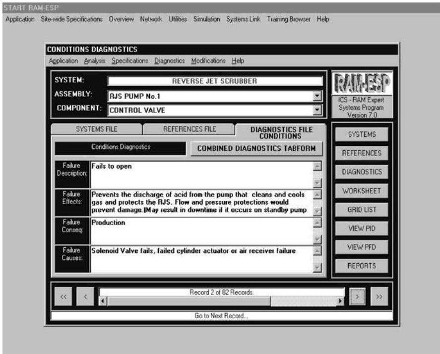
Fig. 3.68 Hazards criticality analysis component condition
